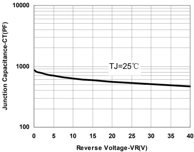
Fig.1-Typical Junction Capacitance
